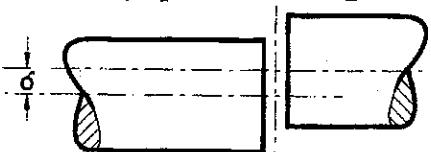
Axial misalignment is present when the axes of the driving and driven shafts are parallel but laterally displaced.
