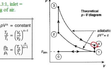
Q11: (cont) Otto cycle; Compression ratio = 8.3:1, inlet = 96.8kPa (abs) at 54°C. Heat supply = 945 kJ/kg of air. (d) Find indicated work (per kg of air).
